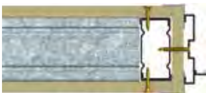
DETAIL B: EXTRUDED ALUMINIUM DOOR JAMB PROFILE
